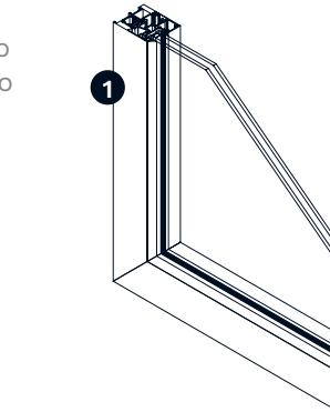
① Aluminum profile with thermal break
